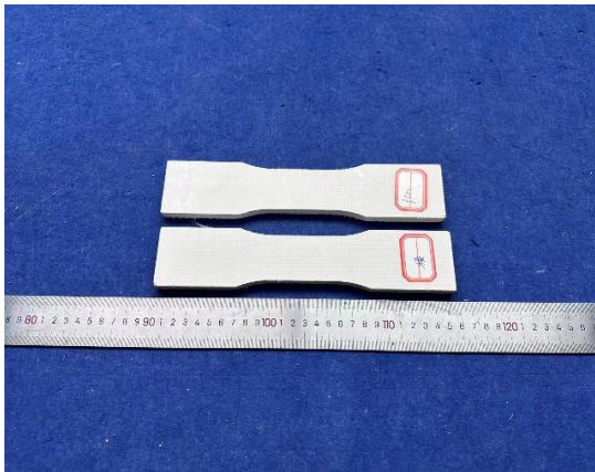
Tension Parallel to Surface - Front view
